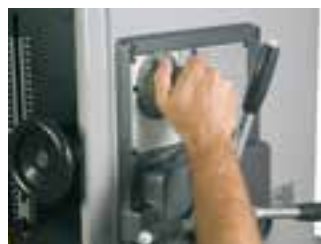
AR 50% lowered feed rate range. Available for A/B/C series.
