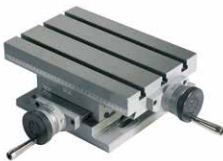
MB1 Cross table. X = 220 mm. Y = 140 mm. Table net weight = 25 kg. Available for EK/T series.
