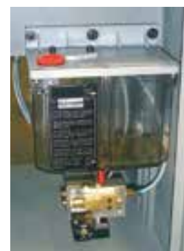
MQL Microlubrication system. Available for all series.
