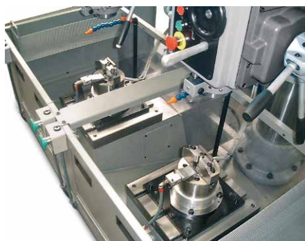
Hydraulic self-centering clamping tools for automation hinge.
