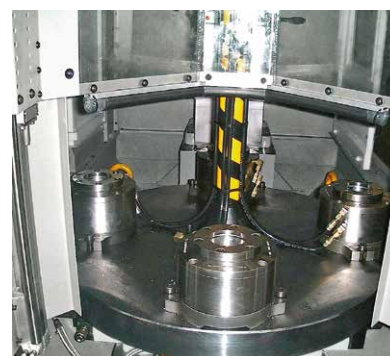
4 Positions rotating table for circular drill battery with synchronized hydraulic clamping tools.
