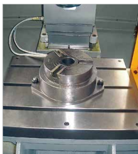
Pneumatic self-centering 3 jaw chuck with synchronized open/close cycle.
