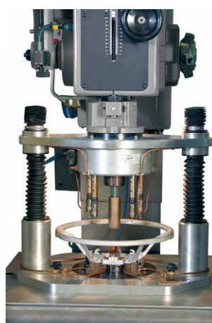
Multi-spindle headstock drilling detail of car handwheels.
