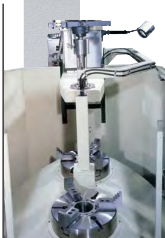
GUIADO HUSILLO PRINCIPAL MAIN SPINDLE GUIDING GUIDE DE LA BROCHE PRINCIPALE FÜHRUNG HAUPTSPINDEL
